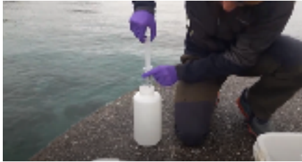
Sample water with syringe
