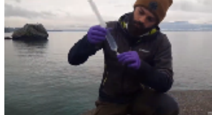
Fix the syringe to the sterivex
