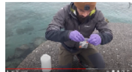
Close the sterivex in the other end and keep it in a plastic bag
